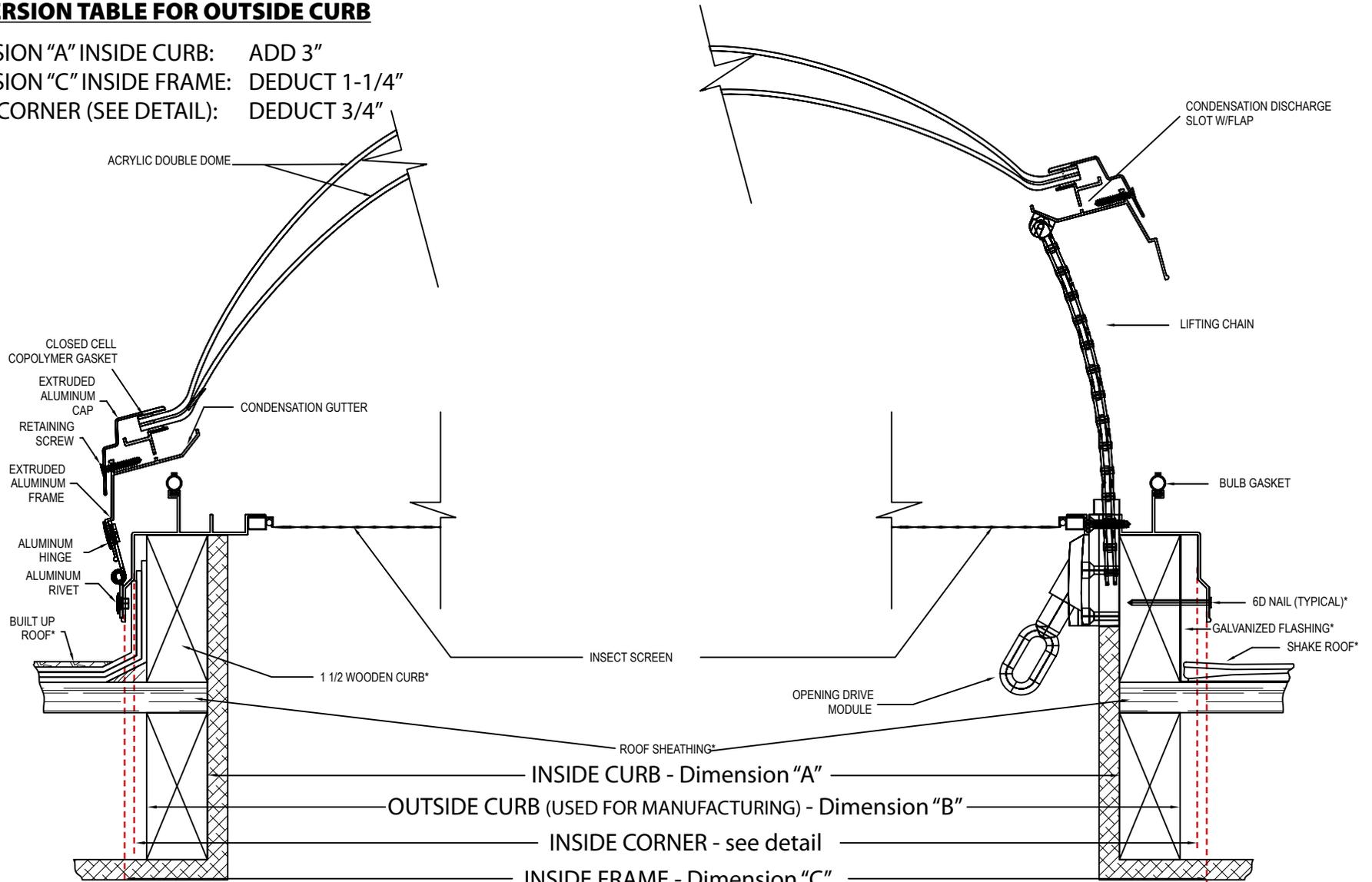
**NOTE: Recommend a minimum 3/12 roof pitch for proper weeping. Flat roof installations NOT recommended.**
